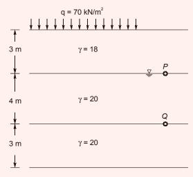
Surcharge (q =  $70 \text{ kN/m}^2$ ) is applied instantaneously hence excess pore pressure (u<sub>i</sub> = 70 kPa) is developed at point P and Q [GWT level is at level P]
