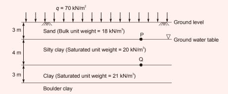
Immediately after preloading, the effective stresses (in kPa) at points P and Q respectively, are
