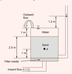
The effective stress (in kPa, round off to two decimal places) at point A, located 1 m above the base of tank, is \_\_\_\_\_.
