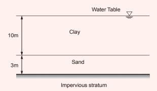
The settlement (in mm, round off to two decimal places) of the clay layer, 10 years after the construction of the fill, is \_\_\_\_\_ (18.83)
