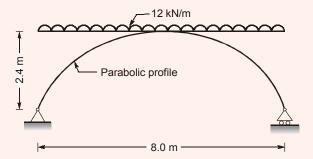
Neglecting self-weight, the maximum bending moment generated in the structure (in kNm, round off to the nearest integer), is \_\_\_\_\_\_.
