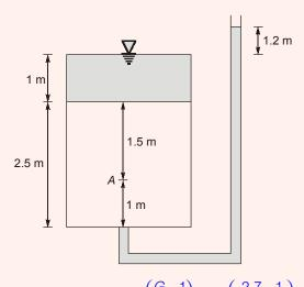
$$\gamma_{suv} = \left(\frac{G-1}{1+e}\right)\gamma_{\omega} = \left(\frac{2.7-1}{1+0.58}\right) \times 10 = 10.759$$
