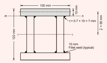
q = Shear stress at the level mn in the weld = 100 MPa =  $\frac{FA\overline{y}}{Ib}$
